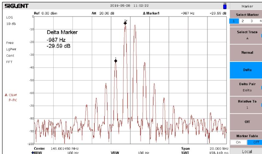
Fig 22: f=145MHz, 7.7Watt PEP, Delta IMD3 = 29,6dB
