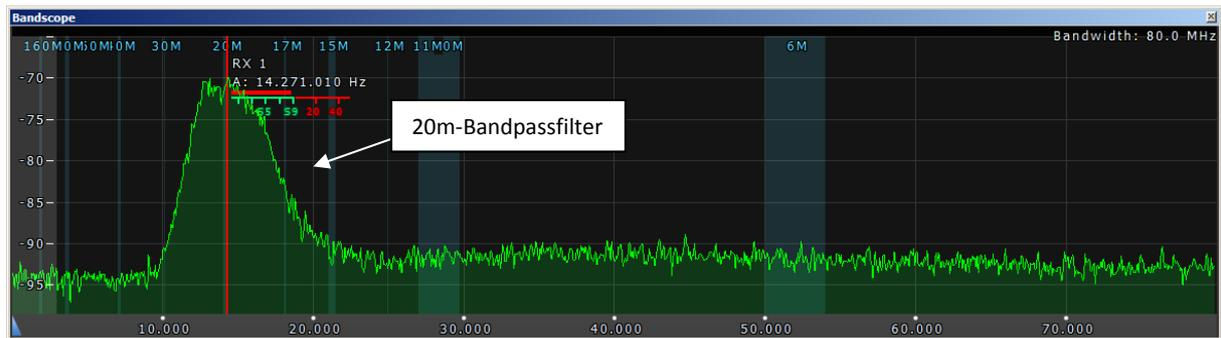
**Figure 16: Spectrum with Wide RX filter off. The receiver now automatically selects a suitable, selective BP filter, in the example at 14.2 MHz in the 20 m band.**
