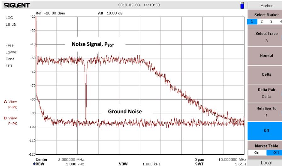
**Figure 13: Spectrum at the input of the receiver. Noise signal up to 5MHz, except in the notch filter**
