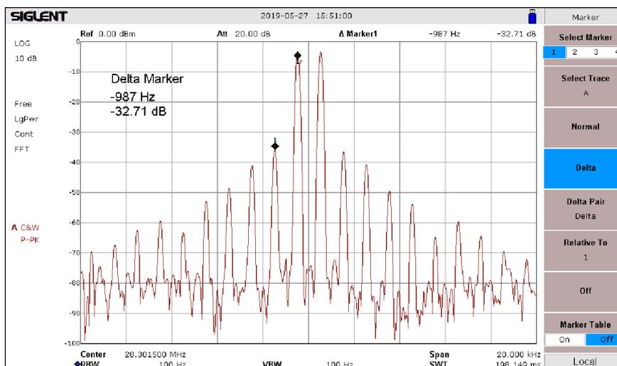
Fig 21:  $f= 28.3\text{MHz}$ , 18Watt PEP,  $\text{Delta IMD3} = 32,7\text{dBc}$
