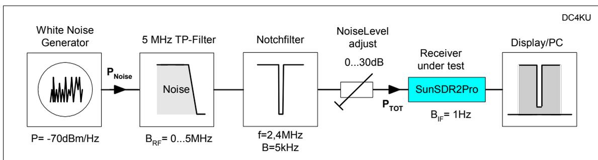
**Figure 12: NPR test setup**
