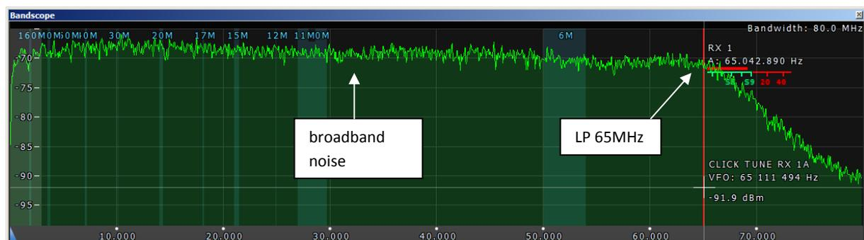
**Figure 15: Spectrum with bandscope and Wide RX Filter on**
