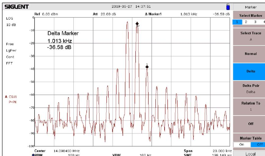
Fig 20:  $f=14,1\text{MHz}$ , 18.7Watt PEP,  $\text{Delta IMD3} = 36,6\text{dBc}$
