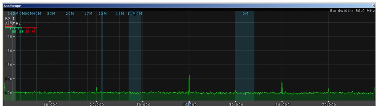
**Bild 17: Receiver Spurious Signals from 0-80MHz**
