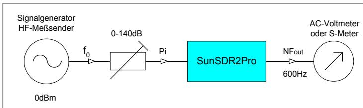
**Figure 4: Test setup to determine the sensitivity**
