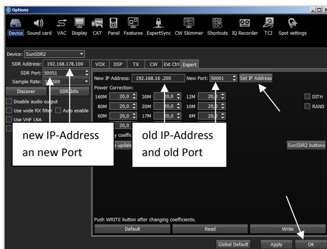
**Figure 6: Changing SDR IP address and port, IP address: 192.168.178.100, port: 50051**
