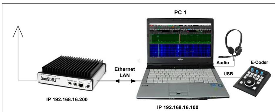
Figure 1: Direct connection to a local PC
