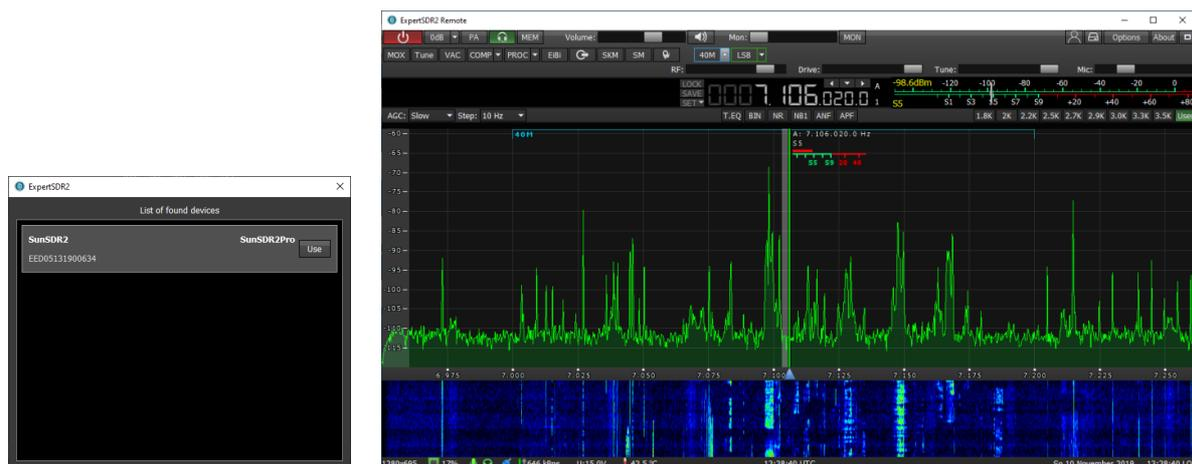
**Figure 14:** SunSDR2Pro is found (left) and can be remotely controlled from the Internet (right)
