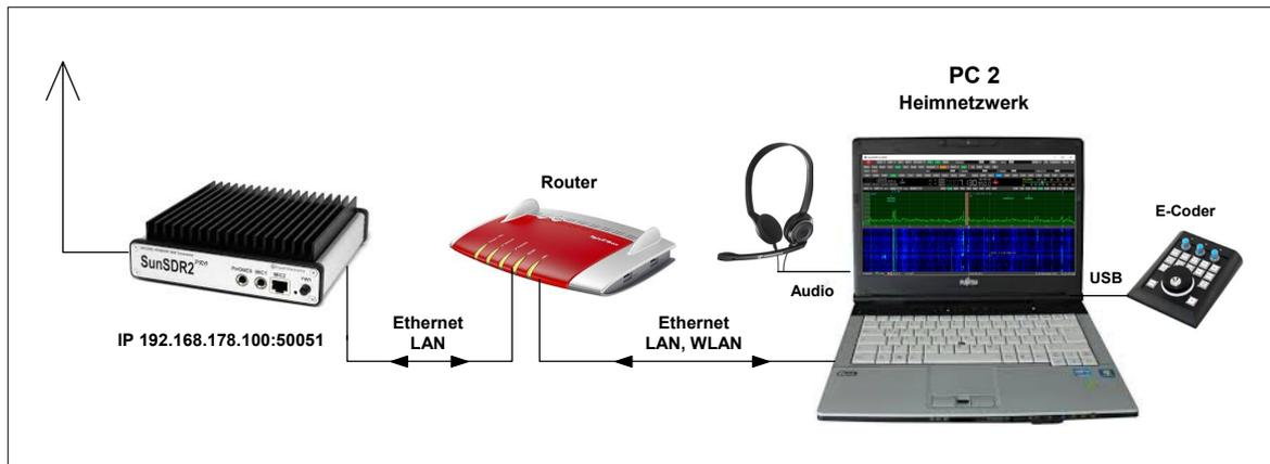
**Figure 5: Connection to any PC in the home network**
