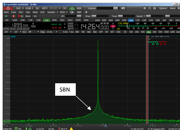
Figure 16: Visible receiver sideband noise at Pi = -10dBm (S9 +63dBm)
