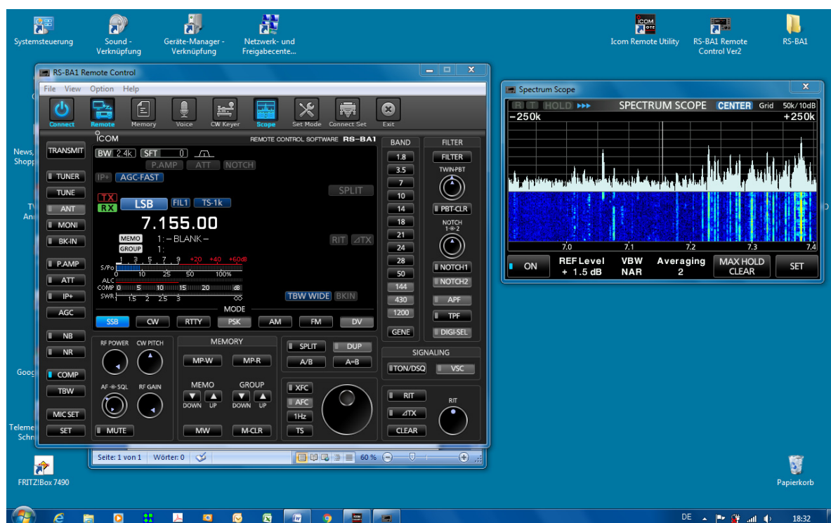
Fig. 10: Remote control of the IC-7300 via a directly connected PC (USB interface)
