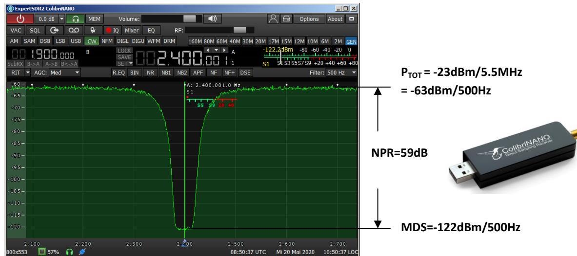
Figure 6: ColibriNANO with  $B_{RF}=5.5\text{MHz}$ ,  $NPR = 59\text{dB}$
