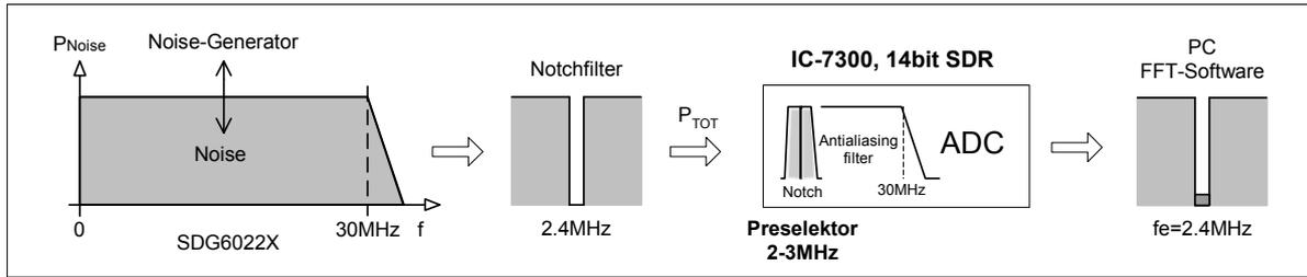
Figure 8: NPR measurement on the IC-7300
