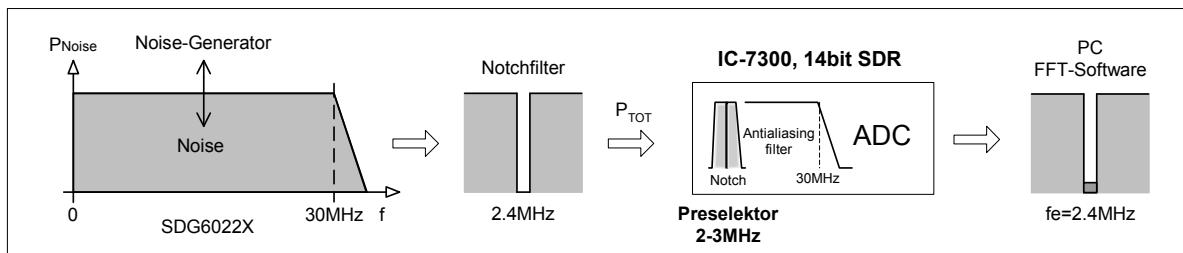
Figure 8: NPR measurement on the IC-7300
