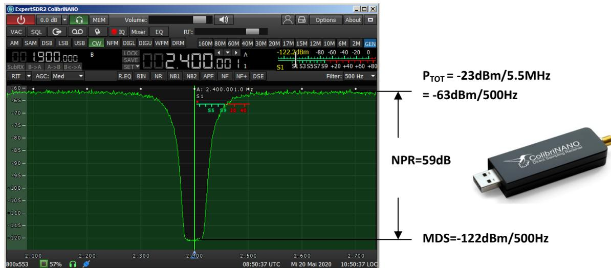
Figure 6: ColibriNANO with  $B_{RF}=5.5\text{MHz}$ , NPR = 59dB
