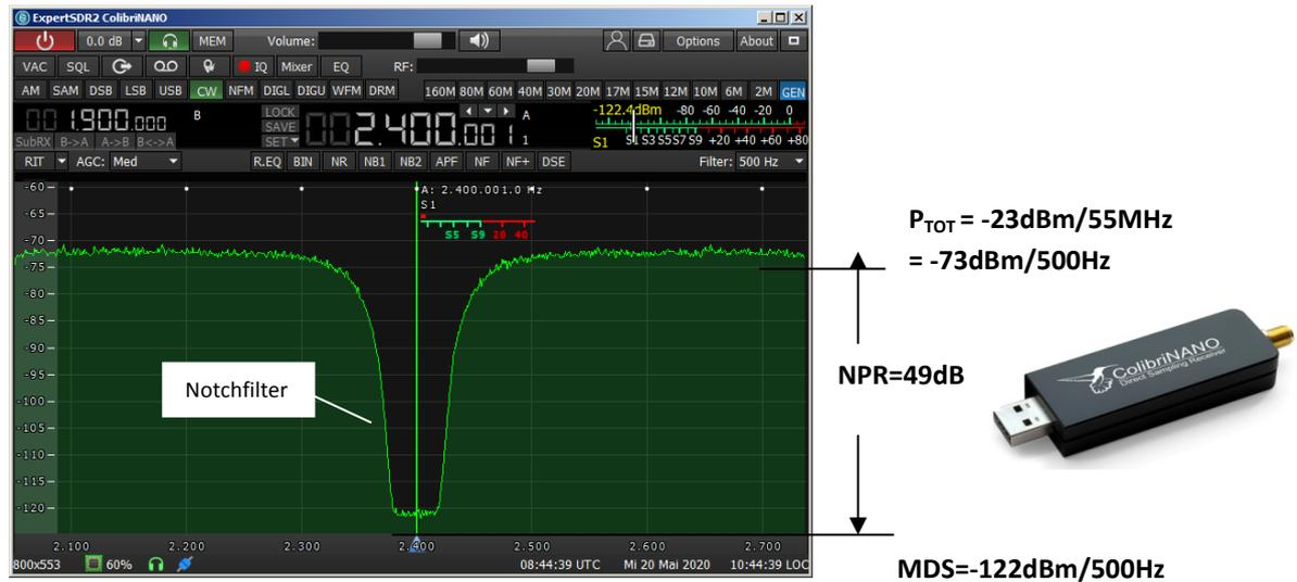
Figure 5: ColibriNANO with  $B_{RF}=55\text{MHz}$ , NPR = 49dB
