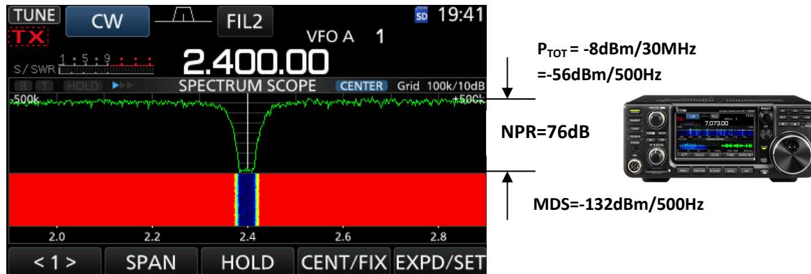
Figure 9: IC-7300,  $\text{NPR} = 76\text{dB}$
