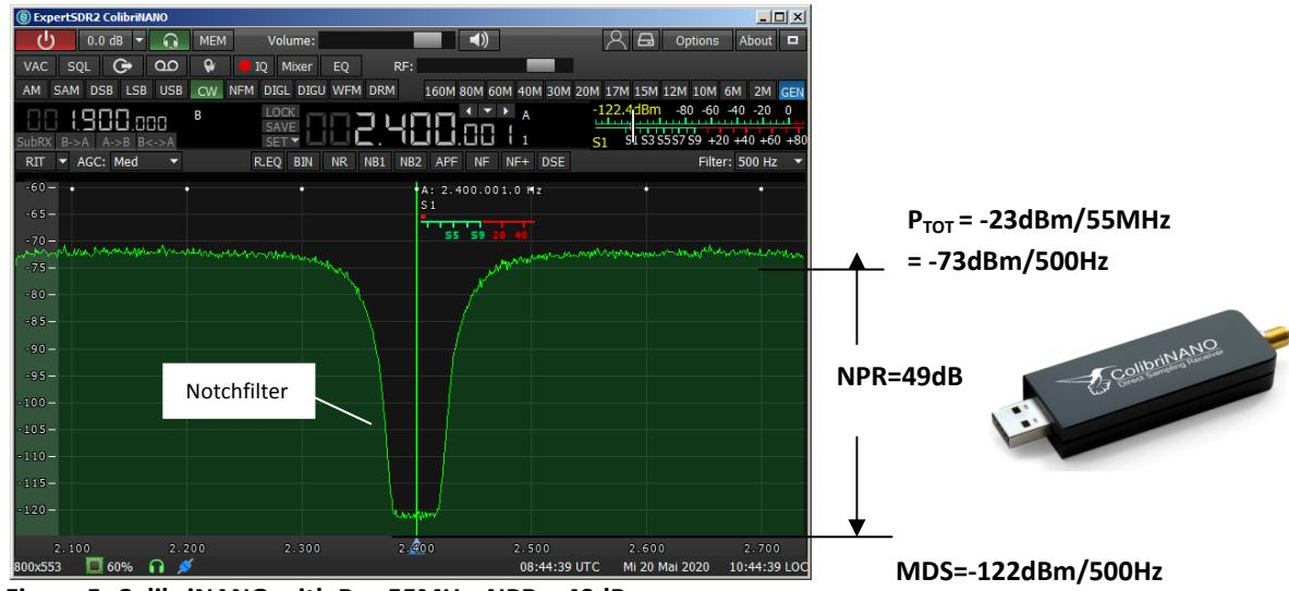
Figure 5: ColibriNANO with  $B_{RF}=55\text{MHz}$ ,  $NPR = 49\text{dB}$
